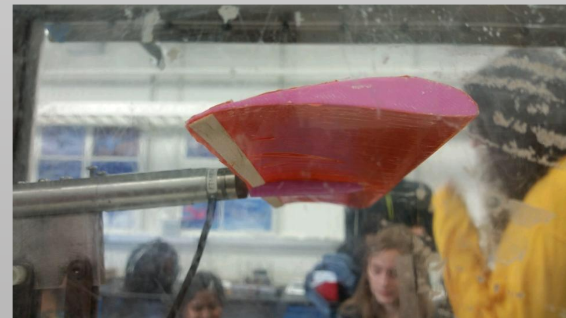
This picture shows the 11" x 4" x 0.5" model wing during a wind tunnel test to determine optimal GF size. The wooden beam at the bottom is the GF.
