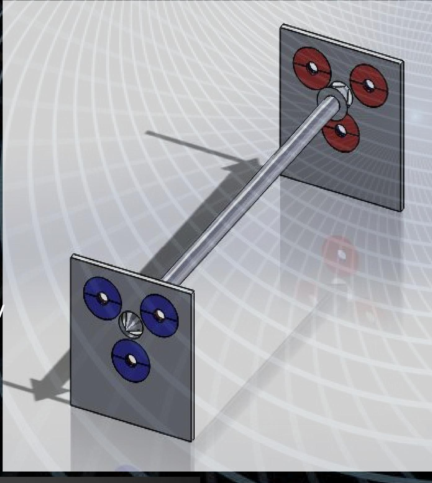
The final design of our project incorporates an alternator at the center of the suspended axle in order to extract rotational energy generated upon its spinning, the error of which we plan to calculate by having the spin initiated by a motor.
