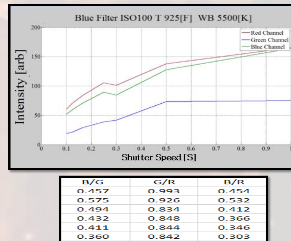
Intensity ratio for ISO 100 and White background. We found multiple linear regions with various slopes.
